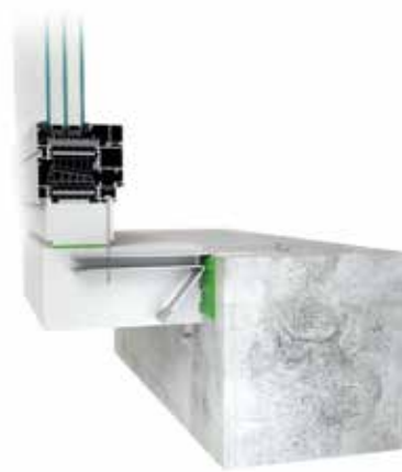
bottom connection, 200 mm beam with internal anchor
